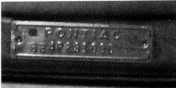
This VIN tag on a 1964 Pontiac LeMans clearly shows it's not a GTO, as the first number is a "6," designating that it was built with the 215-cu.in. straight-six, not a V-8
